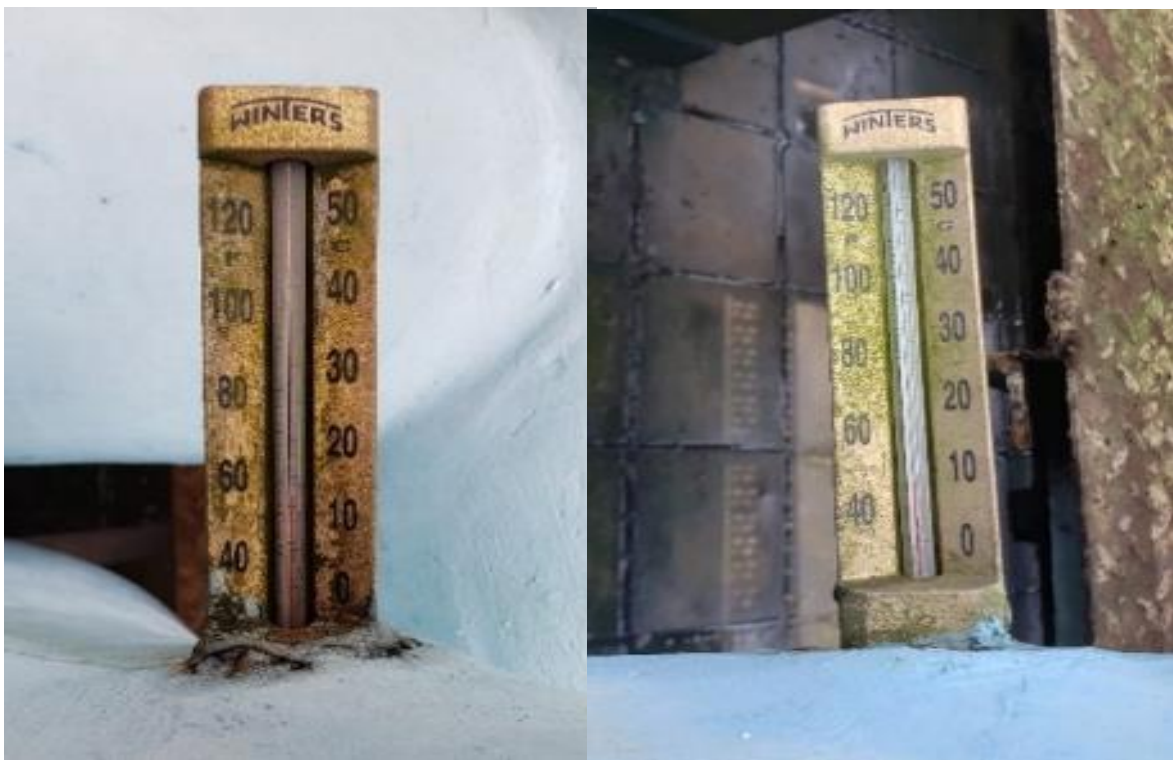
Mercury-in-glass Thermometers with 1°C magnitudes of incremental units
