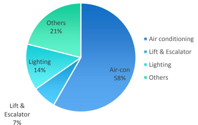
The above breakdown shows that more than half of the total building energy is consumed by the air-conditioning installation. As such, retro-commissioning on the MVAC system is vital for improving energy performance of this building.
